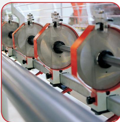
Multi - Cutting Heads Longitudinal multi-cutting heads to cut quilted fabric into stripes
