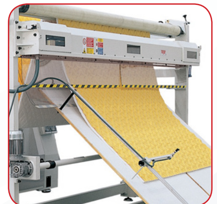
Cross Cutting Cross cutting to cut the quilted fabric into panels
